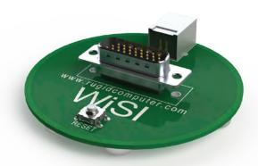
Use a WiSI USB docking station\* to upload and communicate to WiSI nodes from any Windows-based PC.
